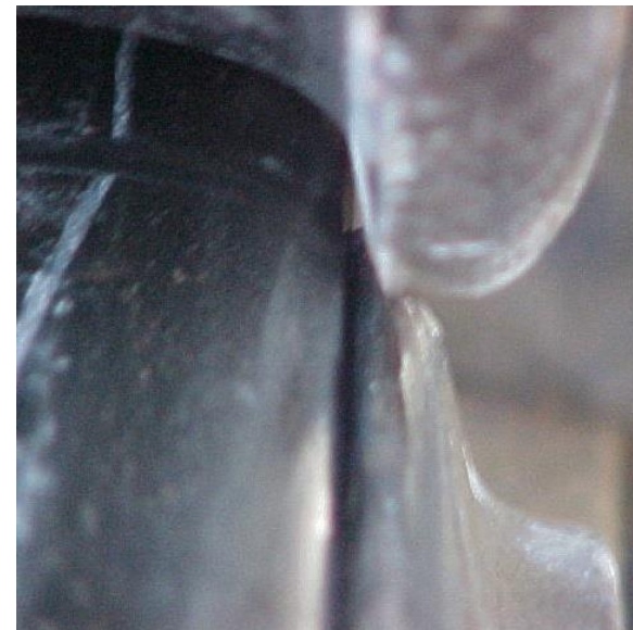
The flange climbs the switch point
