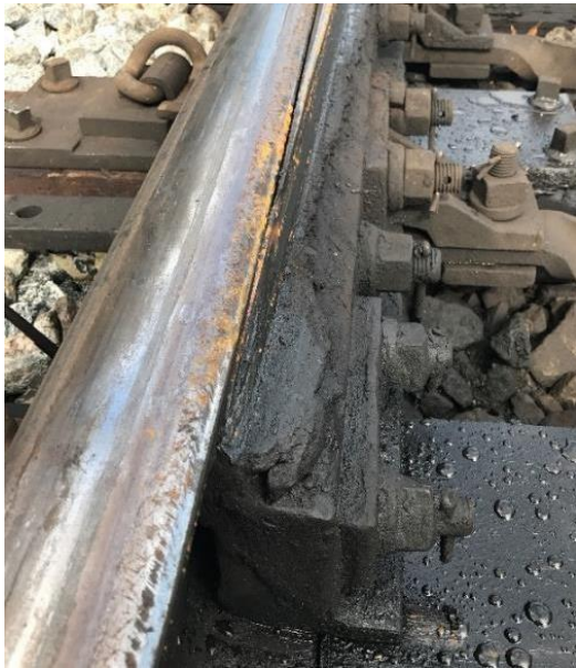
Main track, no. 10 spring switch to a siding, LH diverging point
